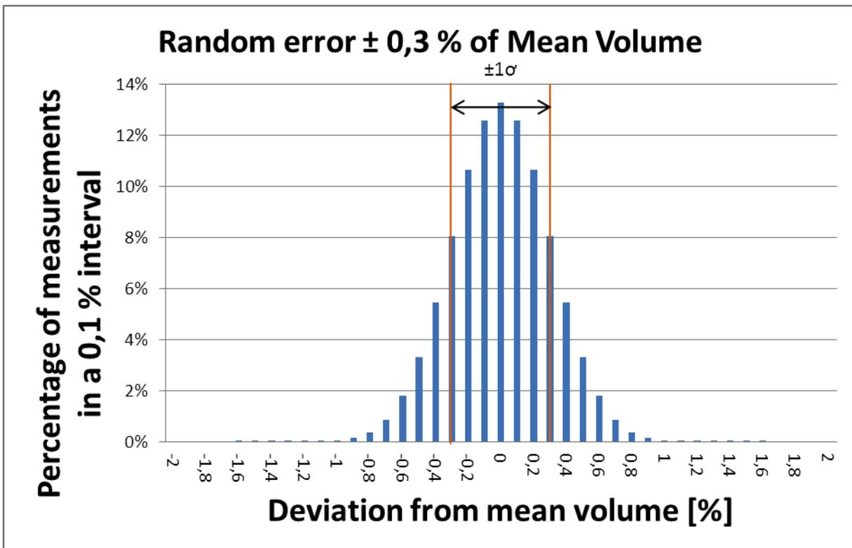
Fig. 4: Measurement distribution for a random error of  $\pm 0,3\%$
