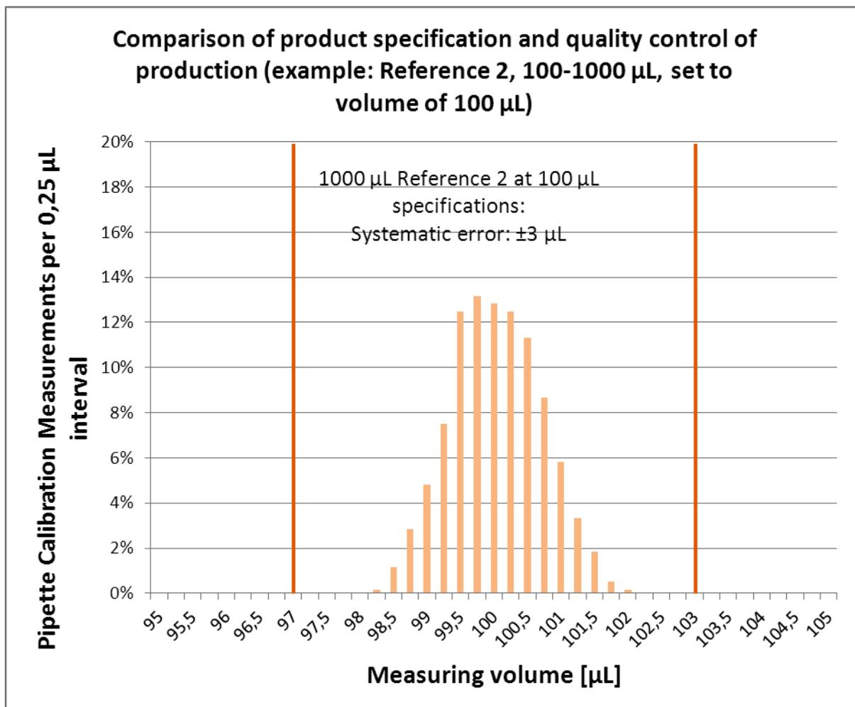
Fig. 7: Distribution of Reference 2 volume measurements (180 individual calibrations)
