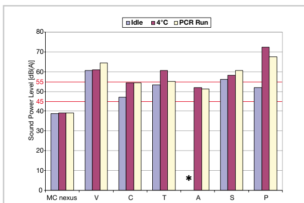
Figure 4: Sound power levels of the thermal cyclers during three operational states. Recommended maximum values according to ISO 11690-1 (see text). (* The fan is switched off in idle state of A. Thus, a relevant differentiation of the operating noise to the surrounding sound level (ca. 32 dB(A)) was not possible.)
