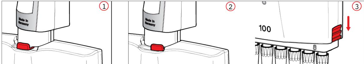
Fig. 5: Opening of the multichannel lower part
