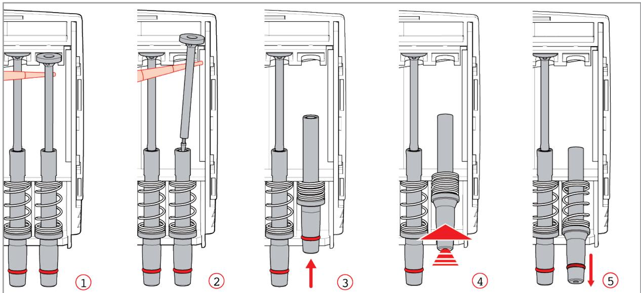
Fig. 6: Removal and installing channels
