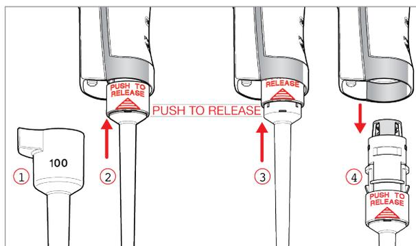
Fig. 4: Removing the lower part
