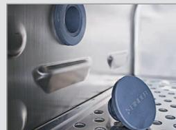
Silicone access port for operating external measuring instruments
